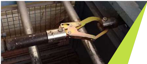
Static Load Testing of Rebar Hook
