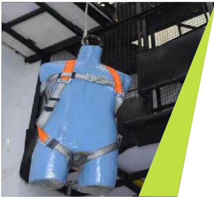
Dynamic Load Testing
