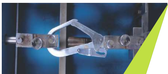
Static Load Testing of Scaffold Hook
