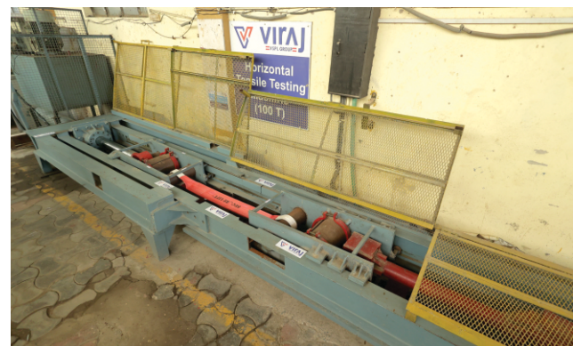
Digital Tensile Testing Machines (100 Ton Max) Sling & Webbing
