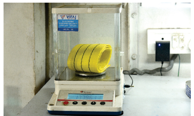
Electronic Weighing Balance (0.001g & 0-220g)
