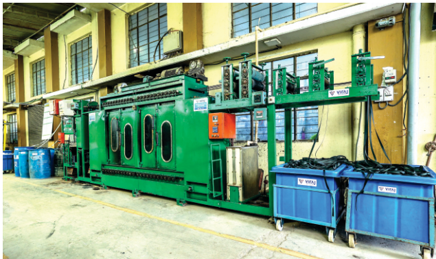
Continous Dyeing M/c for Polyeter (High Temp hot air circulated Process)
