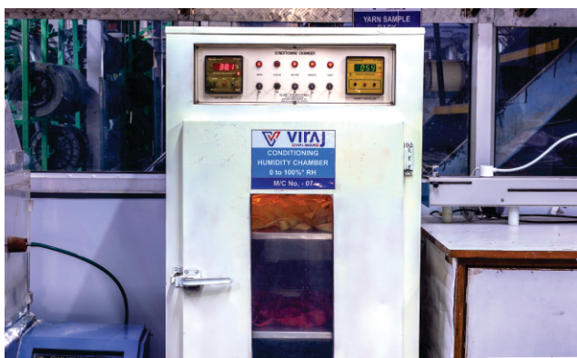
Conditioning Chamber with thermostat Range (0-110 o C)
