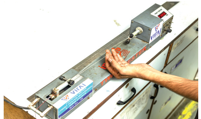
Twist Tester Motorized (0-99999 counts)
